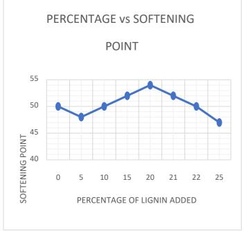
*Figure 2:* Graphical representation of percentage of lignin added Vs softening point values
