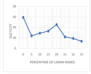
*Figure 3:* Graphical representation of percentage of lignin added Vs ductility values obtained.
