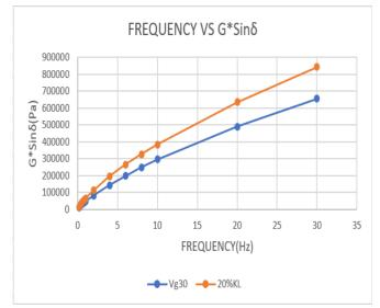
*Figure 4:* Graphical representation of frequency Vs G\*sin delta of Vg30 and 20% LBC binder
