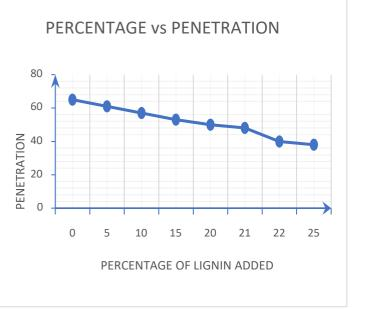
*Figure 1:* Graphical representation of percentage of lignin replaced Vs Penetration Value
