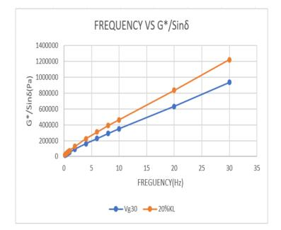
*Figure 5:* Graphical representation of frequency Vs G\*/sin delta of Vg30 and 20% LBC binder
